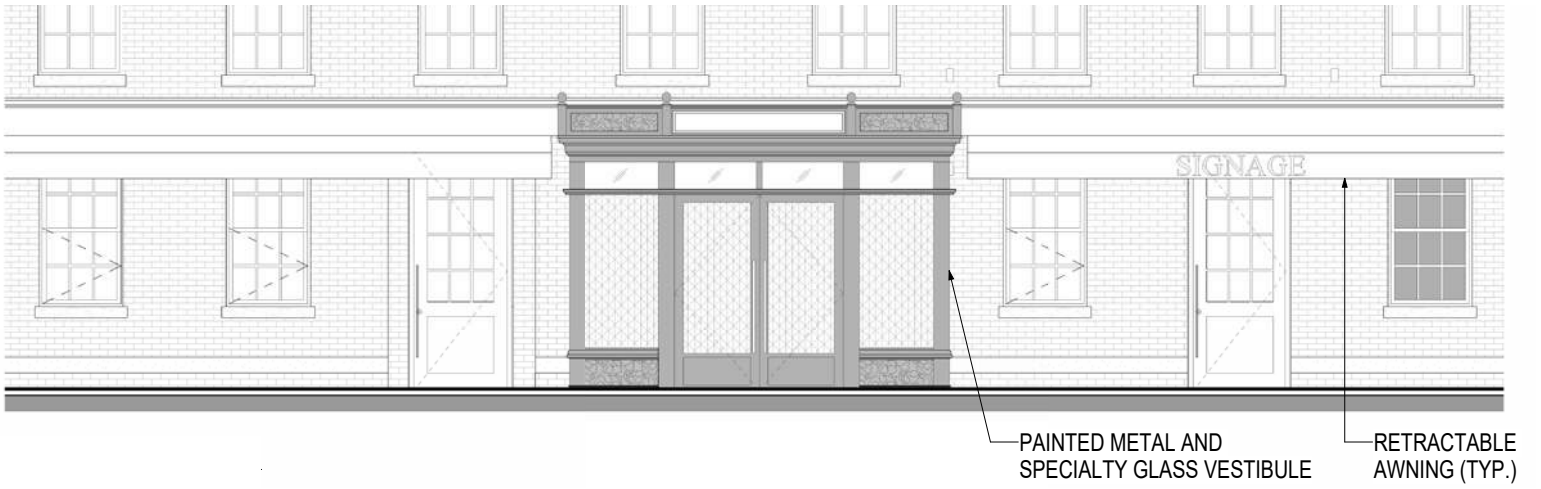
PROPOSED ENTRY VESTIBULE ELEVATION AT 9TH AVE
