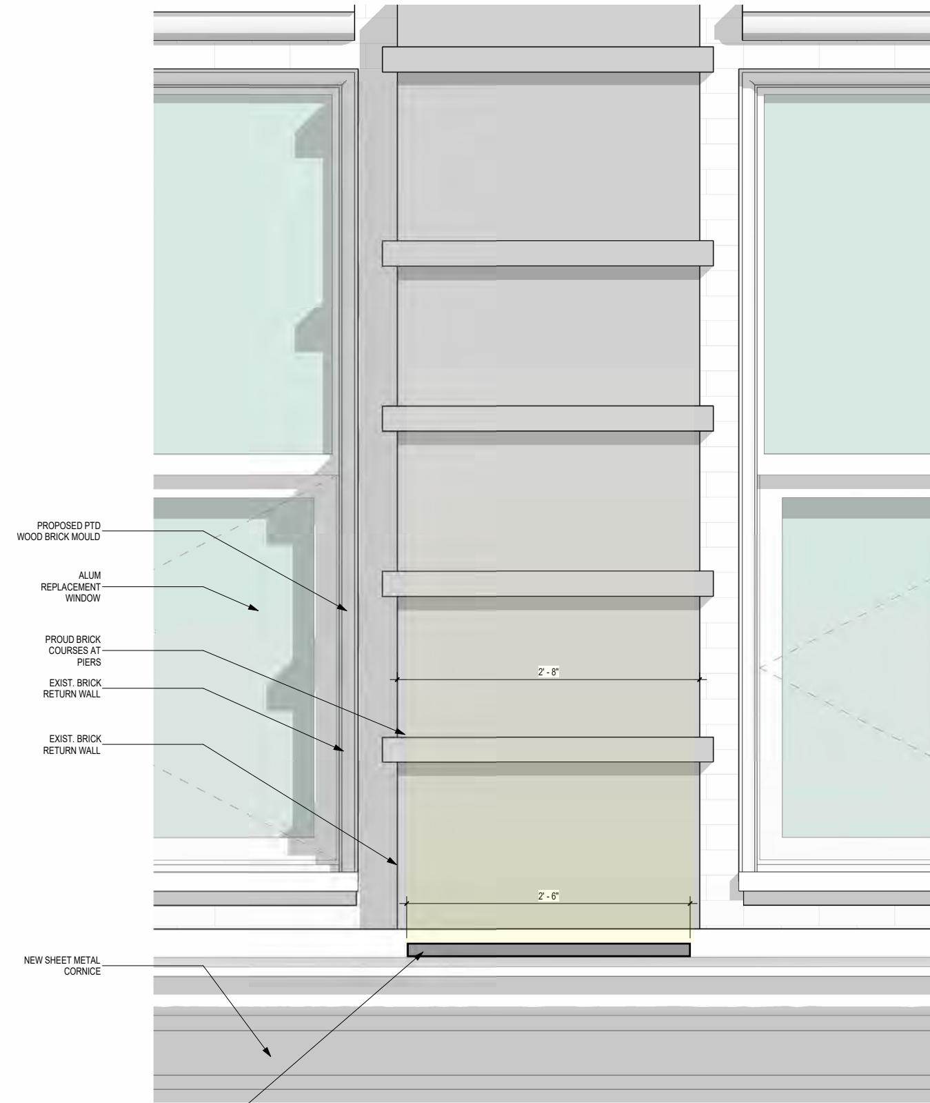
BRICK PIER ELEVATION
