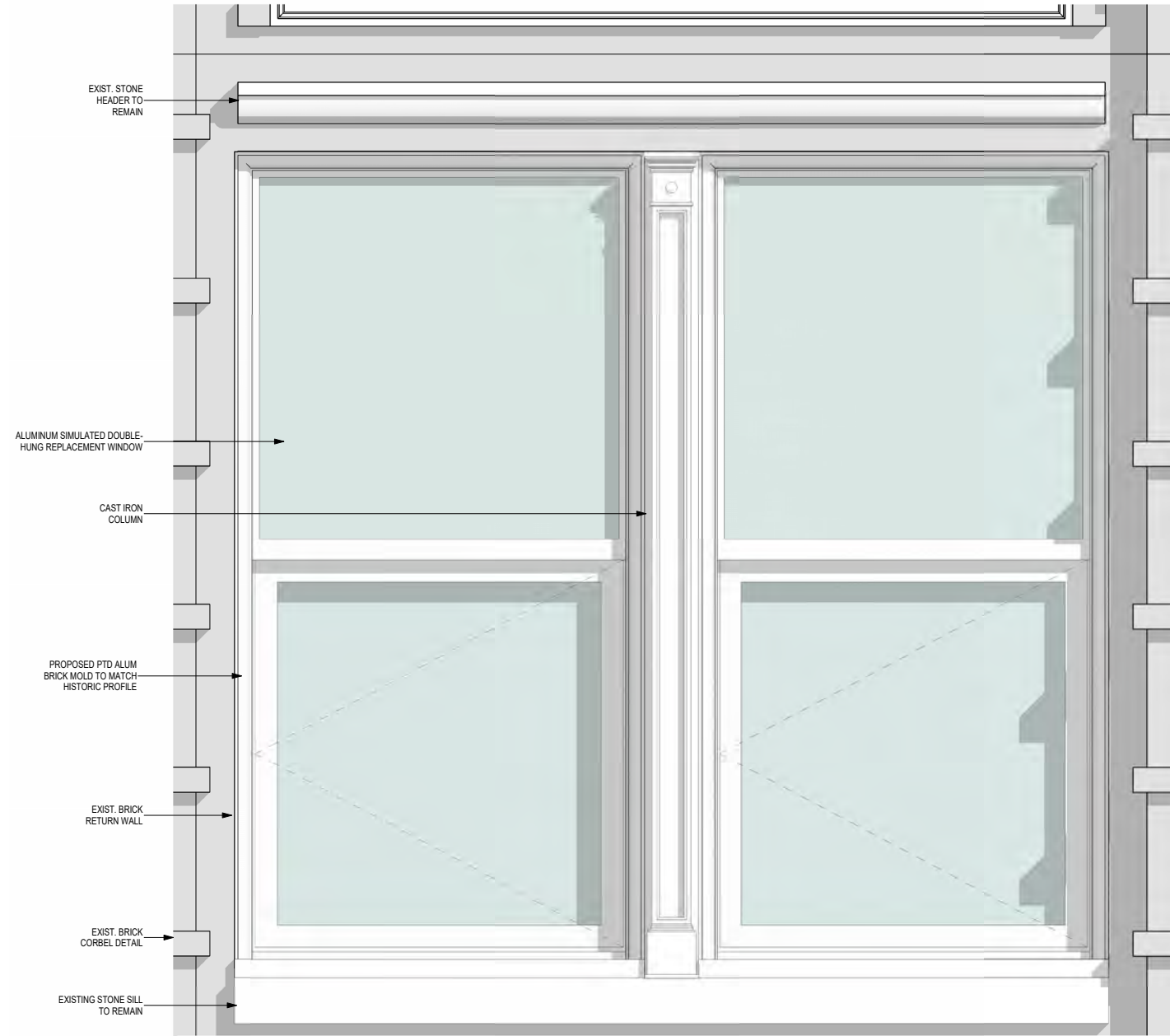
② PROPOSED SIMULATED DOUBLE-HUNG WINDOW 1 1/2" = 1'-0"
