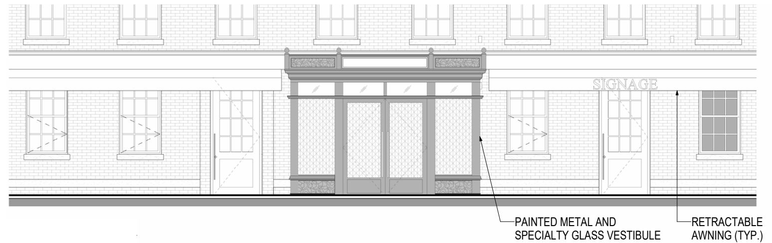
PROPOSED ENTRY VESTIBULE ELEVATION AT 9TH AVE
