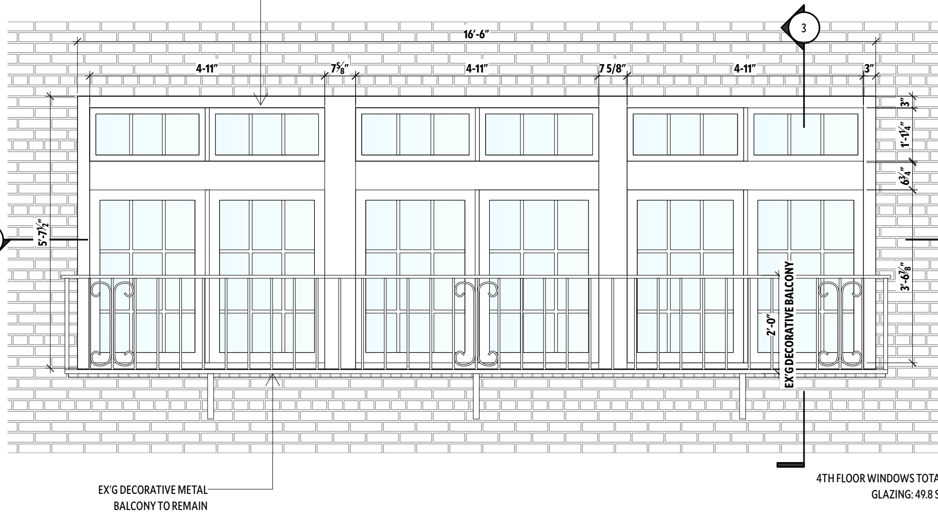
EXISTING ELEVATION: 4TH FLOOR WINDOW 1/2"=1'-0"
