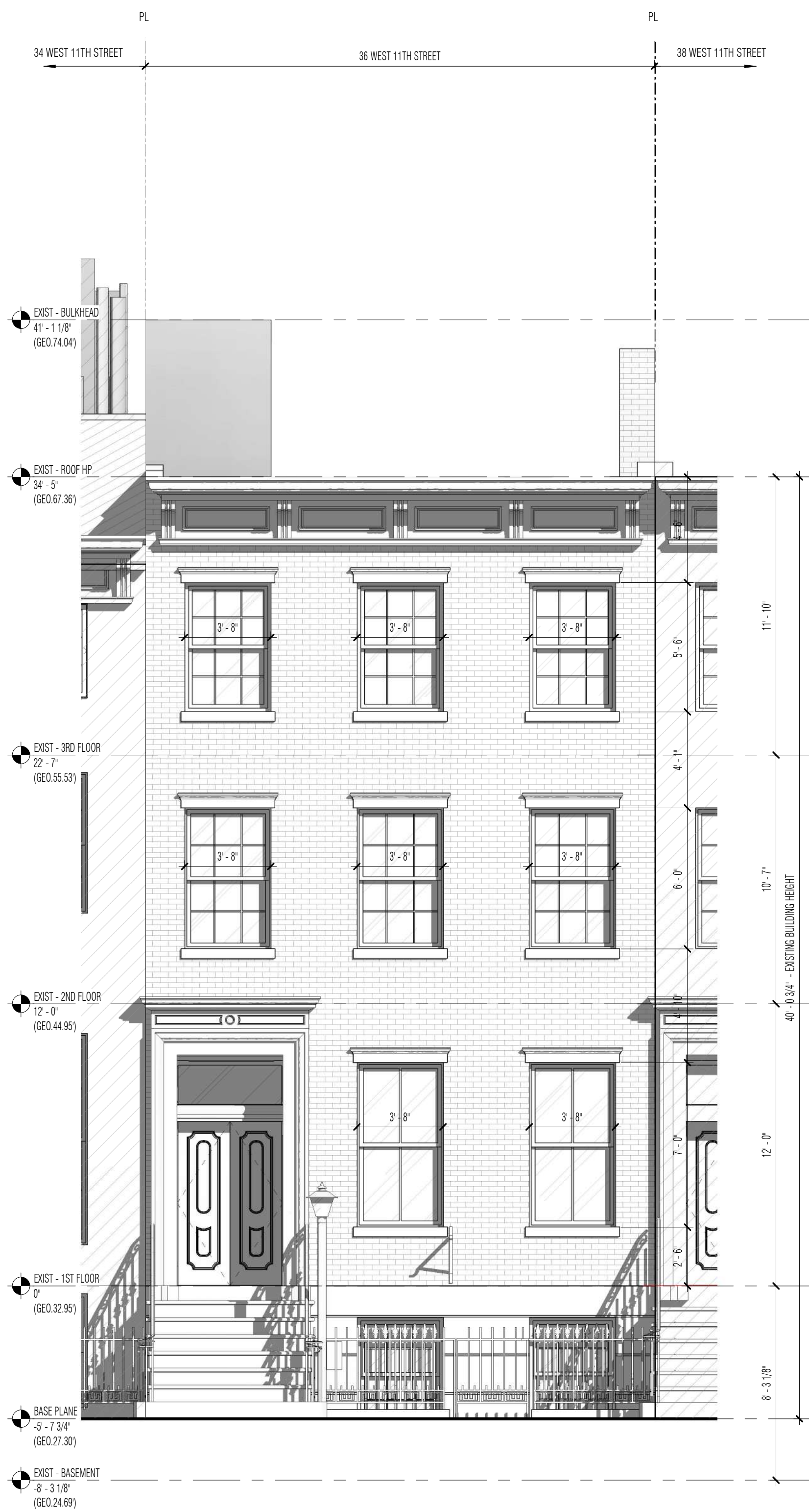
1 ELEVATION - EXISTING STREET FACADE SCALE: 1/4" = 1'-0"
