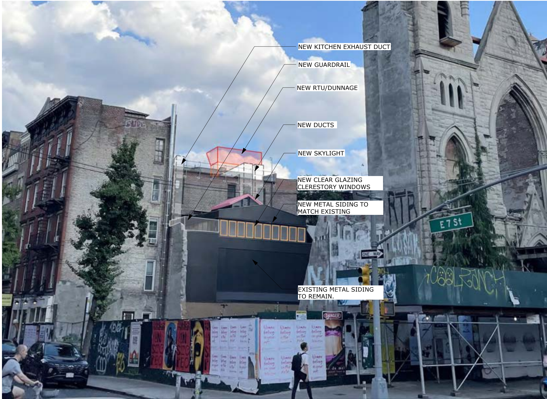
RENDERING OF WEST ELEVATION WITH SUPER IMPOSED RTU AND DUCTS.
