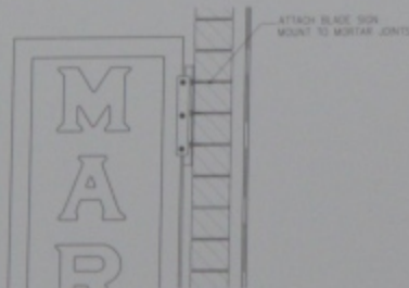
DETAIL OF SIGN ATTACHEMENT
